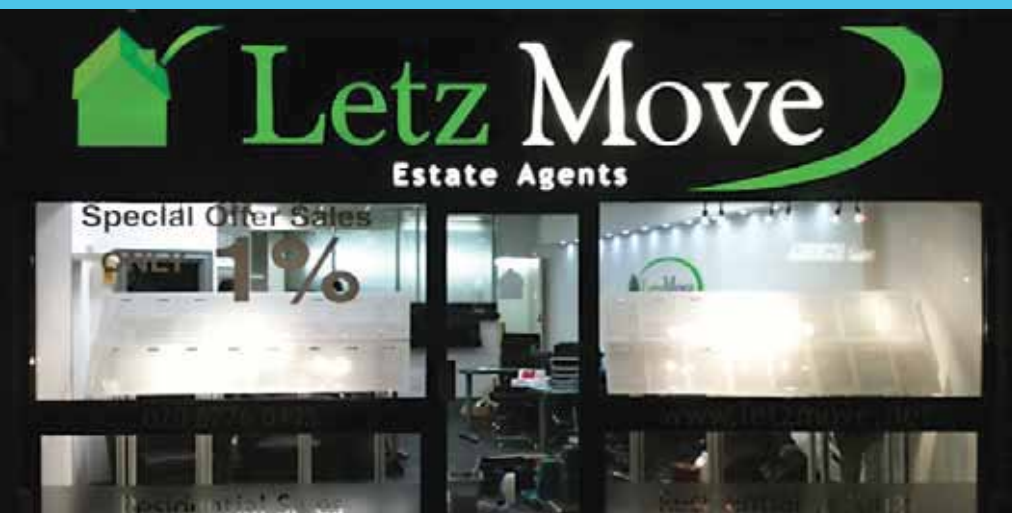
This multi-panel sign features halo illuminated built-up letters
