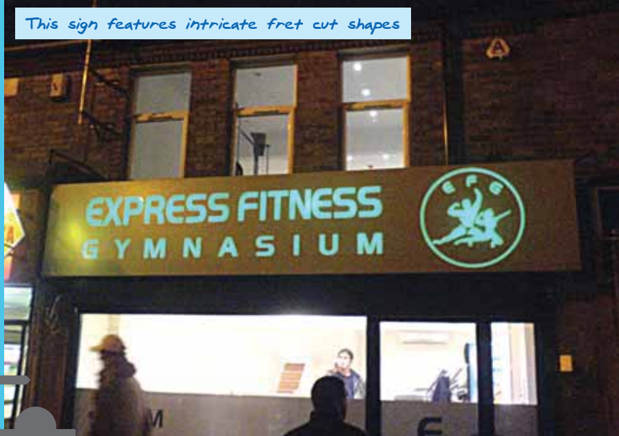
This sign features fret cut illumination and proud letters
